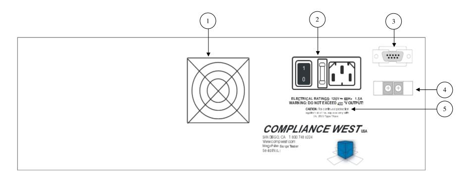
Figure 2. Controls, Indicators, Connectors – MegaPulse Biphasic P EN45502-2-2 Rear Panel
