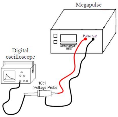
Figure 3. Waveform Measurement Setup
